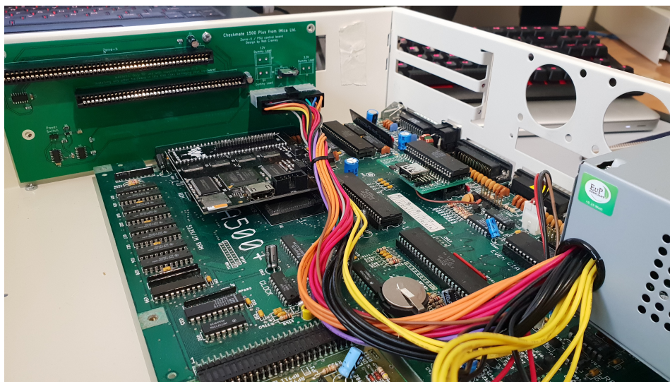
Picture of Zorro board with power cable connected.
