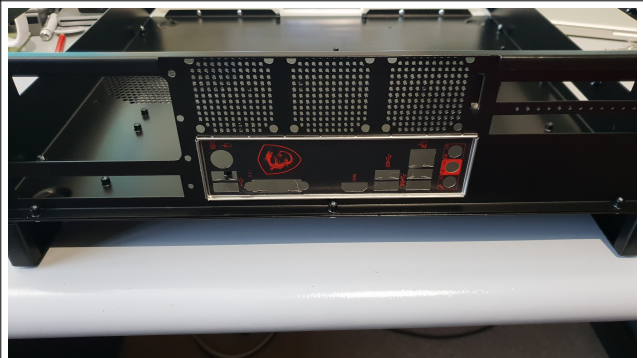
This shows the Motherboard rear port panel fitted into the case rear panel.
