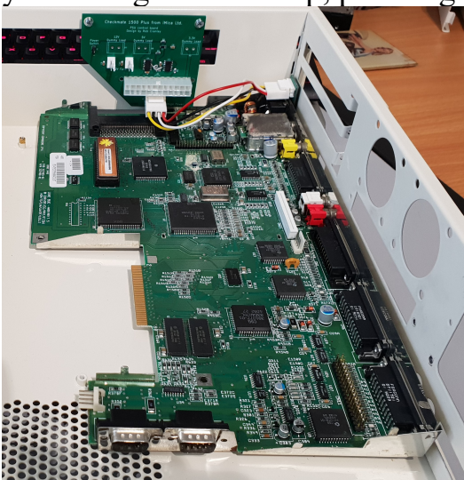
Pictures of A1200 and A600 board's place, note shield should be removed.
