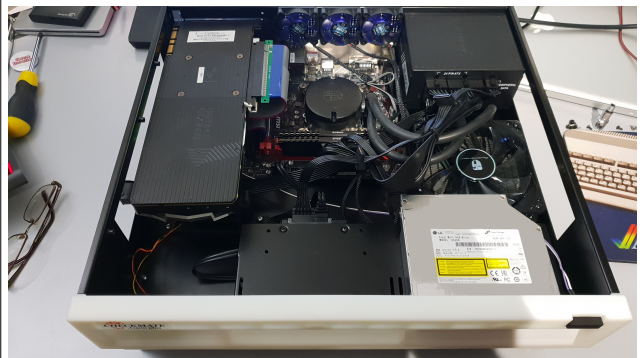
Finished build with GPU fitted, now just mount the lid.
