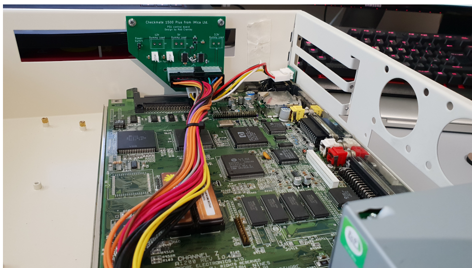
Picture of power adaptor board setup and connected to PSU
