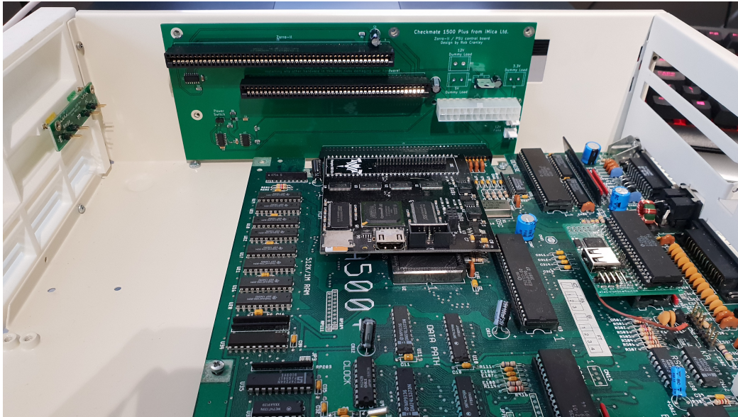
Picture of A500 and Zorro board fixed in place
